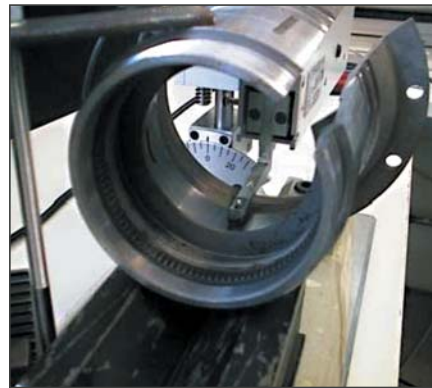
Measuring of a Motor Cylinder Measuring the inside surface of a Rotor
