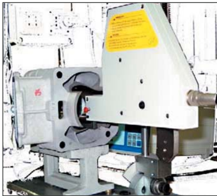
Measuring of a Motor Cylinder Measuring the inside surface of a Rotor
